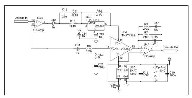
Figure 7. Hifi 2:1 Decoder circuit
