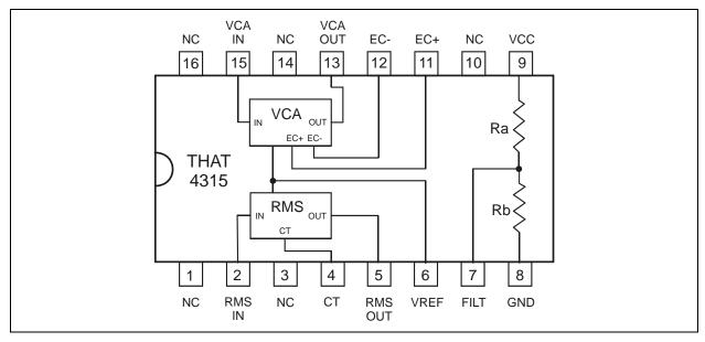
Figure 1. THAT4315 equivalent block diagram
