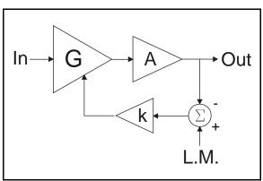
Figure 2. Feedback compressor.
