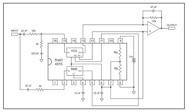
Figure 5. 4315 Typical Application Circuit - 1:2 Expander
