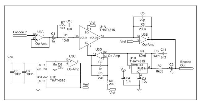
Figure 8. 3:1 Encoder circuit
