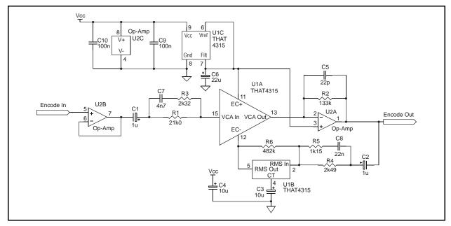
Figure 6. Hifi 2:1 Encoder circuit
