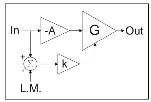
Figure 3. Feedforward expander.
