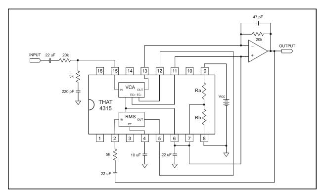
Figure 4. 4315 Typical Application Circuit - 2:1 Compressor
