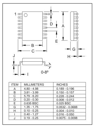
Figure 10. QSOP-16 surface mount package drawing
