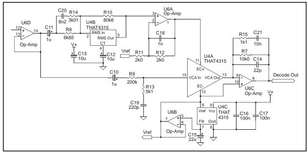
Figure 9. 3:1 Decoder circuit
